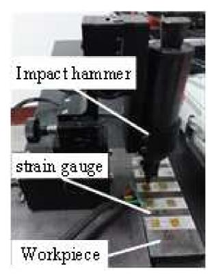
Fig. 3. Residual stress impact device Figure.4 Residual stress measurement of the scene
