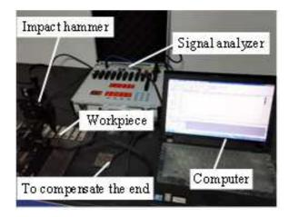
Fig. 4. Residual stress measurement of the scene
