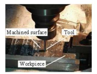
Fig. 2. The milling test scene
