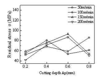
Fig. 6. Cutting speed - cutting depth on the influence of residual stress(f=0.04mm/z, Ae=8mm)
